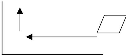
If “External” the tool will lift off from the part as shown.
